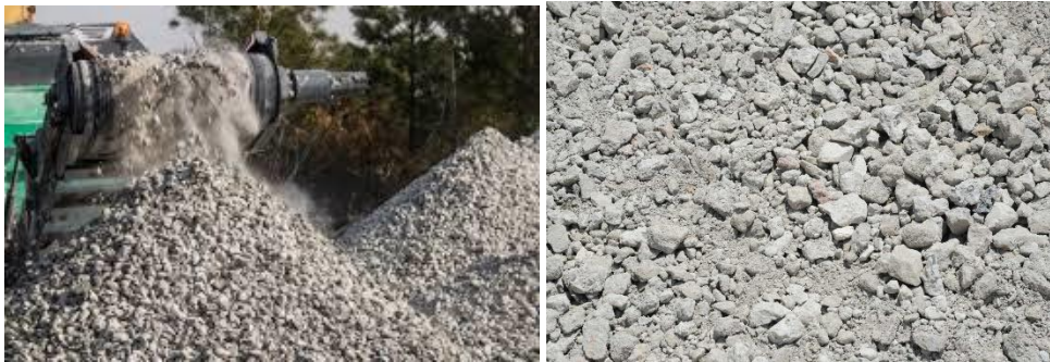
Figure 20: Concrete reprocessed into coarse or fine aggregates
