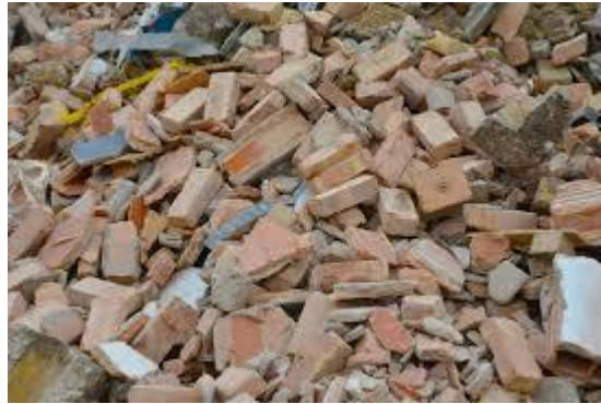
Figure 21: Clay bricks from demolition waste
