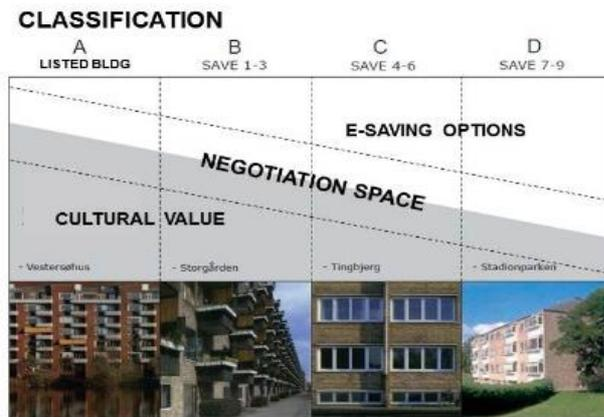
Figure 10 Illustration of the relation between the historic building category and the amount of energy saving that is possible in the buildings (Note: this is only an example not a fixed correlation) [3Encult D.2.3/3.2]
