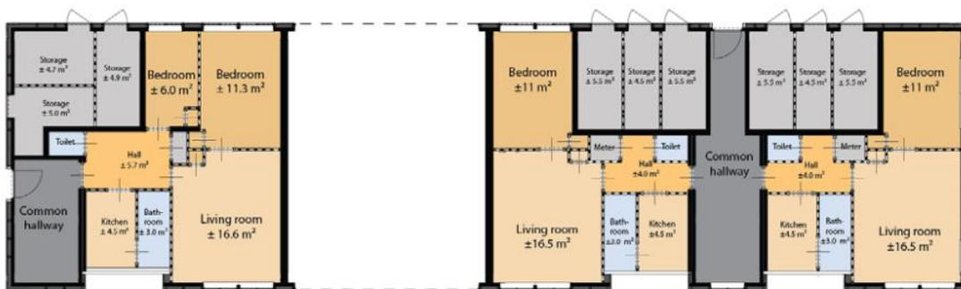
Figure 31 Ground floor with apartments of the Airey-buildings. (Hooyschuur) Source: Kist b2016
